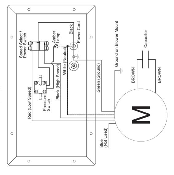
H1990M Control Panel Wiring Diagram
