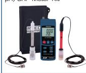
Includes: R3000SD Data Logging pH/ ORP Meter, R3000SD-PH2 General Purpose Electrode, & R3000SD-ORP Professional ORP Electrode
