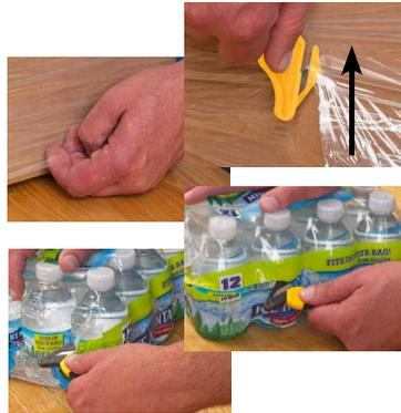
**Tip:** Start the cut from the bottom of the material and pull up toward the top of the pallet. Keep material taut while cutting.
