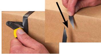
**Tip:** Klever safety cutters are not designed to cut metal banding.
