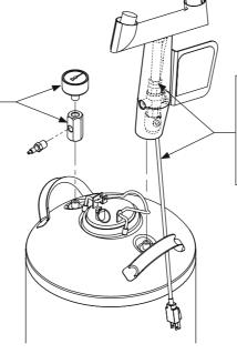
Attach the eyewash yoke assembly to the tank. Max. torque 150 In-Lbs. Route the cable through the tank handle.
