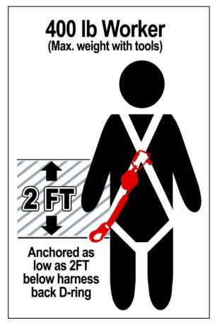
• The TurboLite and Twin Turbo System external shock-absorber (on the lifeline) can deploy up to approximately 12-inches.
