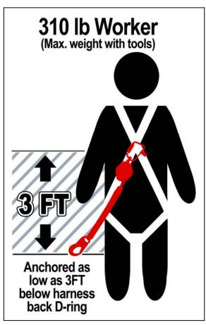
• No other shock-absorber is needed for either the TurboLite or Twin Turbo System. The external shock absorber (on the lifeline) does not deploy.
