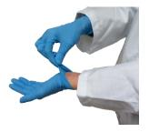
3. Fold the glove completely on itself so that the inner surface is reflected on the outside. Once the first glove removed, hold it with your gloved hand. The contaminated surface is now located inside the glove.
