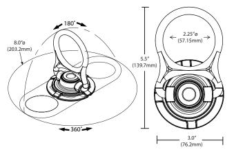
Tensile Strength (UTS): 5,000-lbf (22kN)
